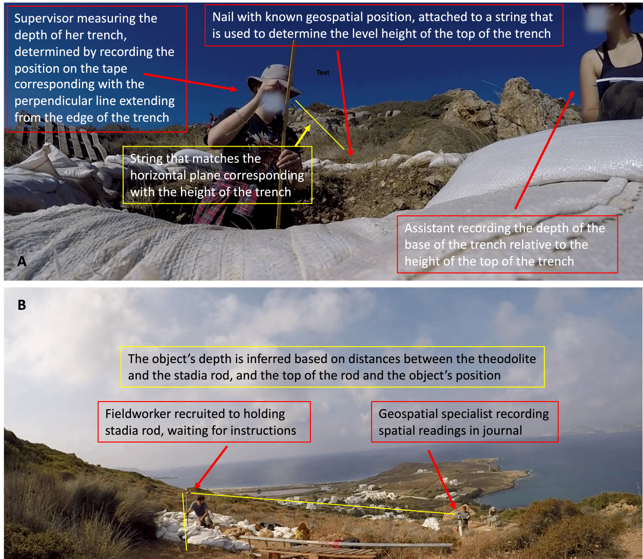
Figure 5: Recording spatial information in the field. A depicts a system that measures distance in relation to trench entities. B depicts a geospatial specialist and a fieldworker determining an object's position using a digital theodolite.
